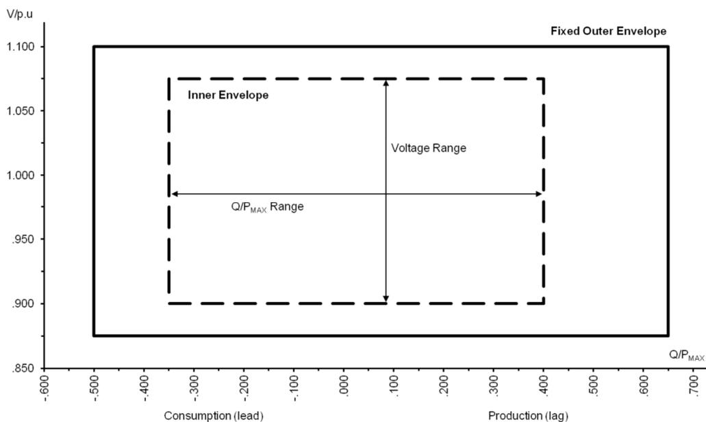
**Figure 5 - Typical U-Q/Pmax-profile of a power generating module (ENTSO-E NC Requirements for Generators)**
