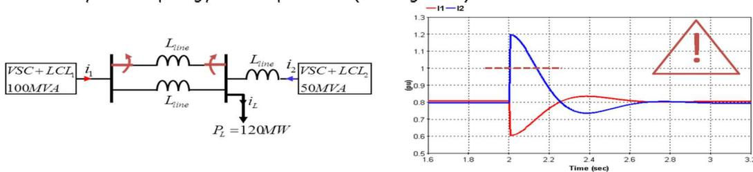
**Figure 7 – Potential PE overload due to uneven load sharing**
