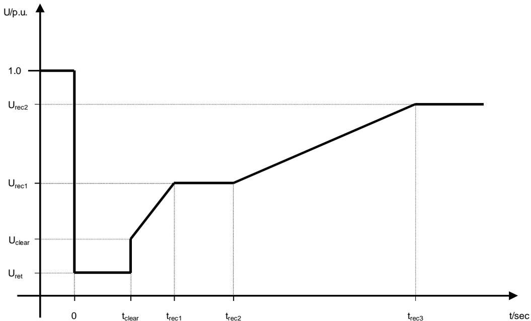
**Figure 6 - Typical FRT profile of a power generating module (ENTSO-E NC Requirements for Generators – Article 14)**
