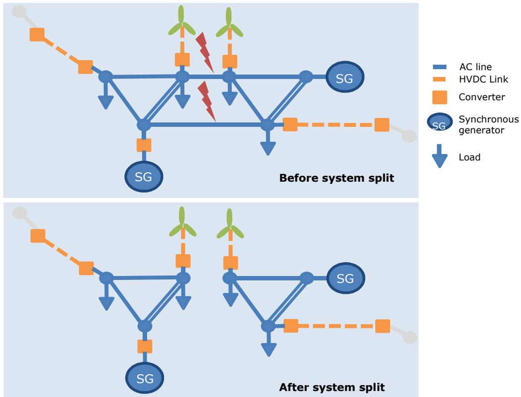
Figure 8 – Example of system split leading to a system with 100% PE
