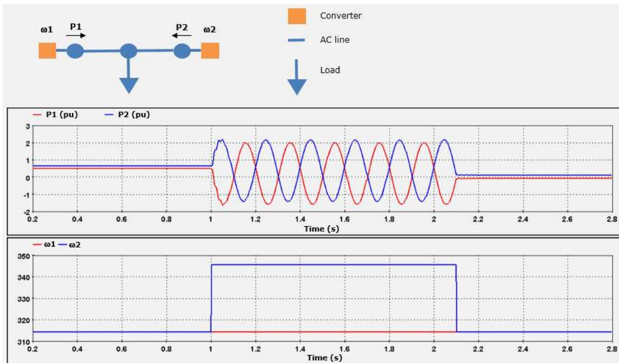
*Figure 3 – Power swings induced by non-uniform steady-state frequencies*
